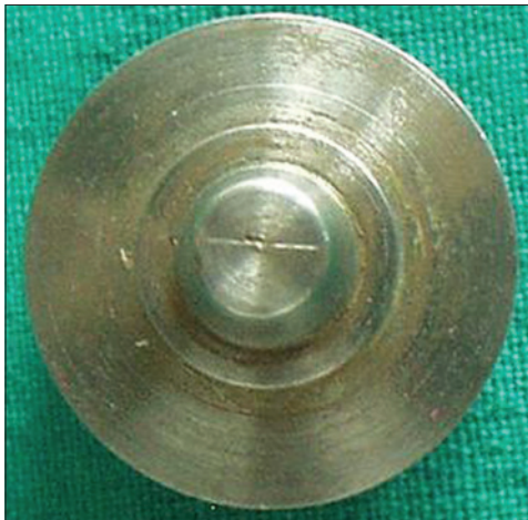
Figure 2: Steel master die: Showing vertical groove
